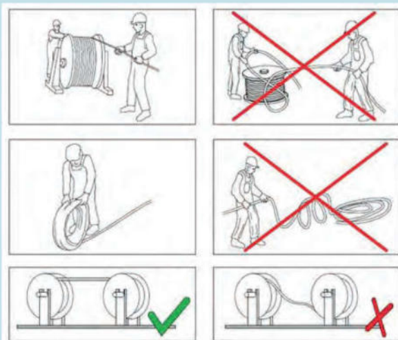
Proper handling of hoist ropes; Schindler rope installation manual
