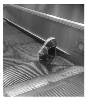
the top and bottom of the flight. If an object approaches the handrail entry or becomes caught between the handrail and entry portal, the safety switch will actuate to stop the escalator. The function of the handrail-
